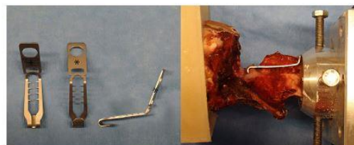
Figure 2 Photographs of the dorsal atlantoaxial instability (AAI) clamp and after fixation on a specimen. *Corresponds to the application component of the clamp that is snapped off after placement.
