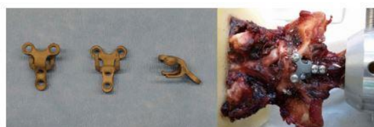
Figure 3 Photographs of the ventral atlantoaxial instability (AAI) hook plate and hook plate after fixation on a specimen.
